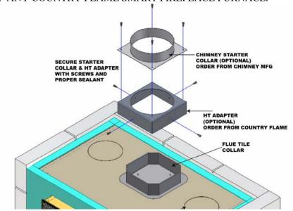
FIGURE 6: TYPICAL HT ADAPTER (optional) INSTALLATION
